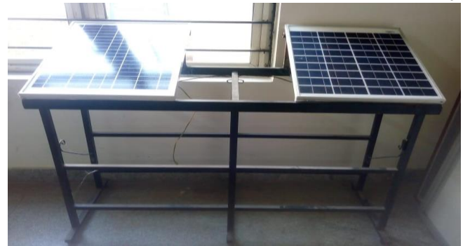
Figure 2 Assembly of solar PV test system
